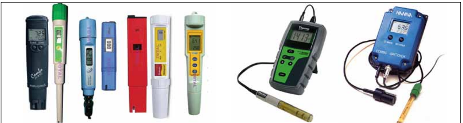
Pictured are various stand alone pH and EC meters and combo meters that do both pH and EC at the lower to medium end of the price scale.
