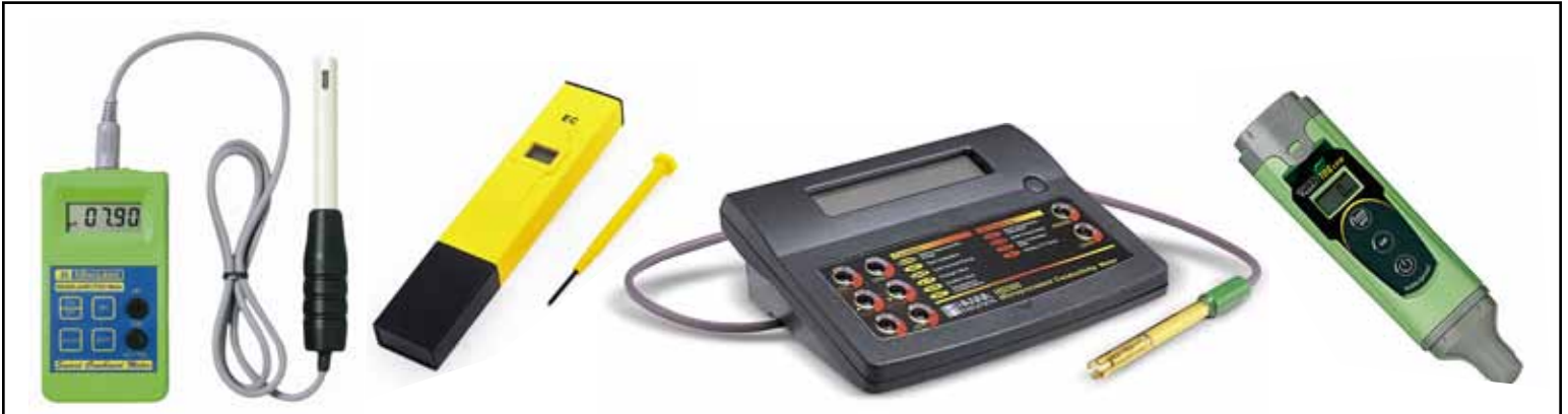
An assortment of different manufacturers EC meters- EC meters are made to measure fertilizer solutions. TDS meters measure total dissolved solids and were originally designed to check drinking water not nutrients.
